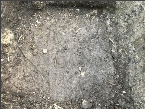
Clogged geotextile on top of the aggregate (Note that the geotextile is flat across the top)
