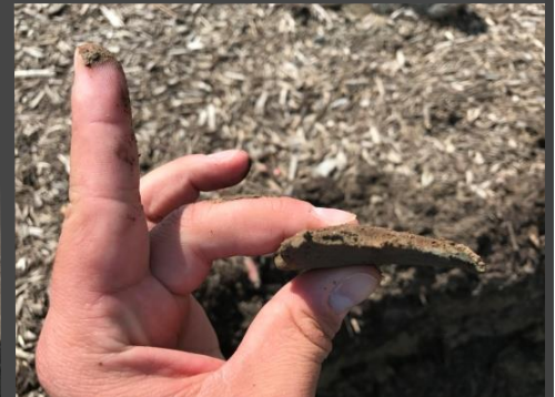
Thick deposits of clay and silt found on top of geotextile
