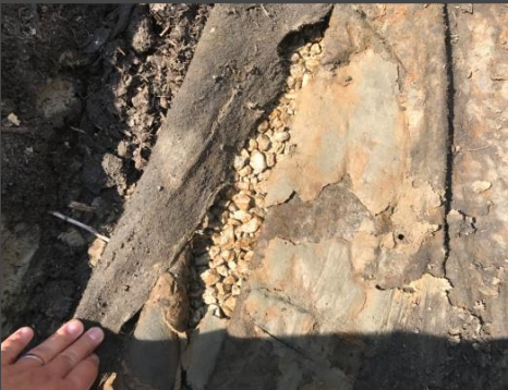
Clogged geotextile on top of the aggregate (Note that the geotextile is flat across the top)
