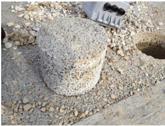
Figure 3-21. Eight-Inch Core Removed for Inserting Monitoring Wells with Temperature Sensors at Various Depths into Porous Pavement Surface.
