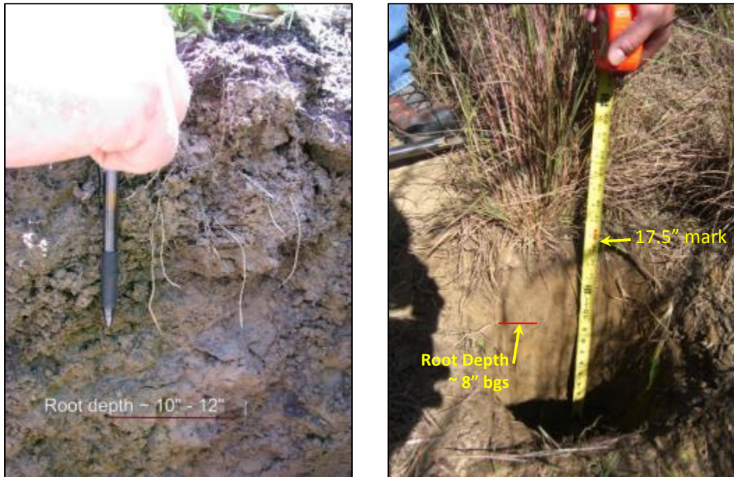
Figure 4-2: Root growth in uncompacted native soil (left) and compacted native soil (right)
